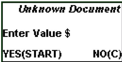
Enter banknote denomination \$ value using the numeric numbers (0-9) on the control panel [for example, for \$5 bill, press numeric key 5 and for \$10 bill, press 1 + 0 keys and so on]
