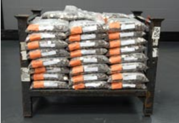
The plastic bags are stacked on the pallet with all labels facing out.
